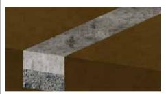
Fill concrete, 3 parts sand + 1 part water + 1 part cement, into the base of the trench.
